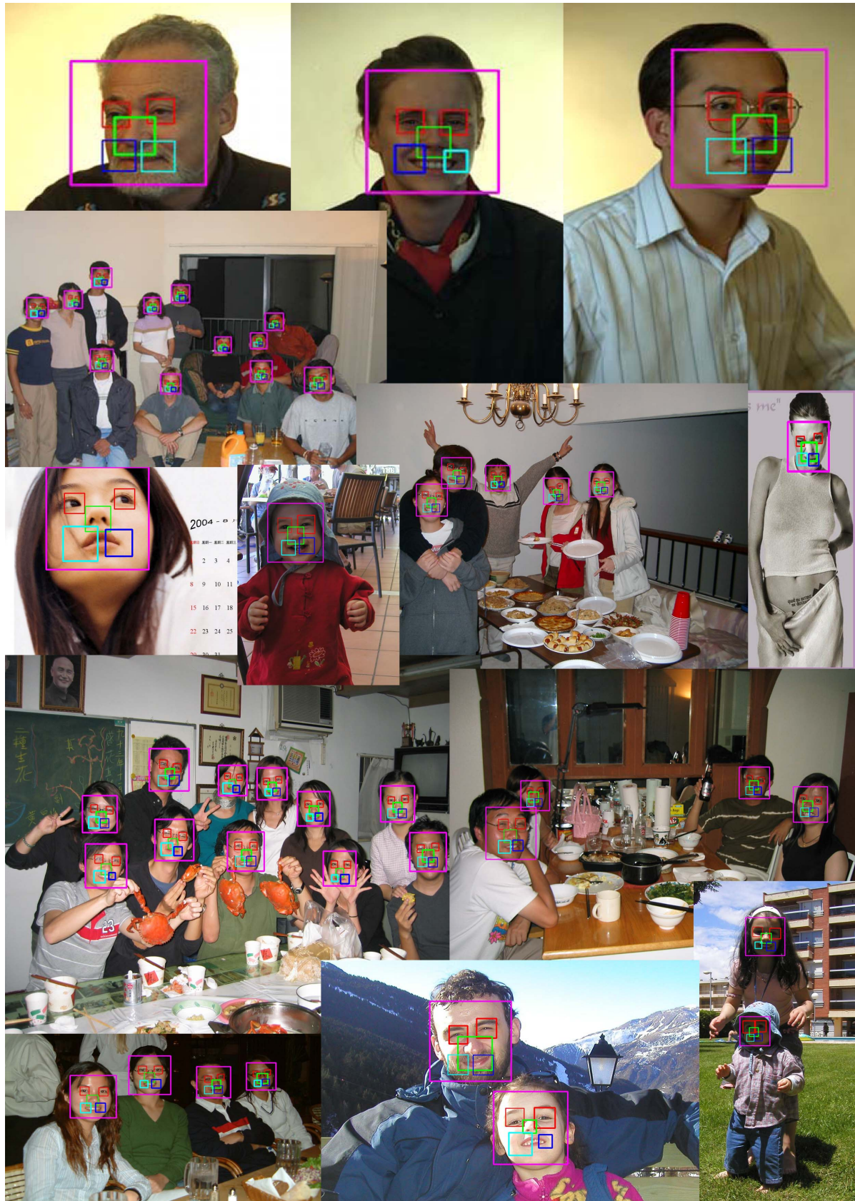
Figure 5. Visual output of our facial component detector from Feret and our consumer photograph testset. Each face is marked by a pink rectangle. Eyes, nose top, left lip corner, and right lip corner inside each face are marked by red, green, light blue and dark blue rectangles respectively. The challenges for the detection include varying pose, outdoor illumination (directional lights and shadowing, expression, wearing sunglasses, and low resolution (small) faces.
