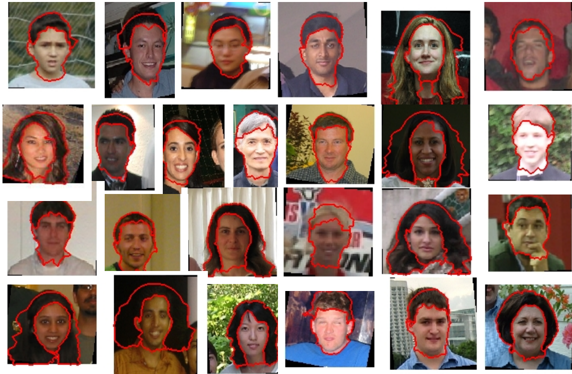
Figure 6. Hair and face segmentation results on low resolution images by our proposed LBP Algorithm.
